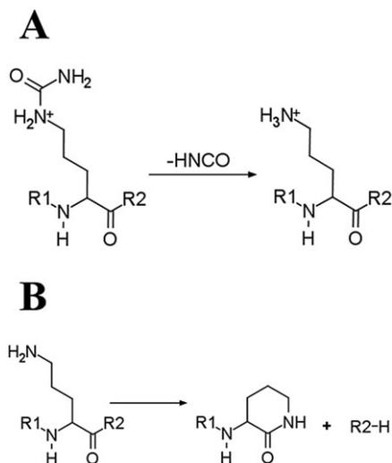
**FIGURE 2** Proposed mechanism for citrulline effect leading to facile cleavage C-terminal to citrulline residues for protonated peptides in the gas phase. First step: loss of isocyanic acid (HNCO) characteristic to citrulline residues, leading to an ornithine residue (A).<sup>8</sup> Second step: cleavage of the Orn-Aaa bond (B)<sup>12</sup>
